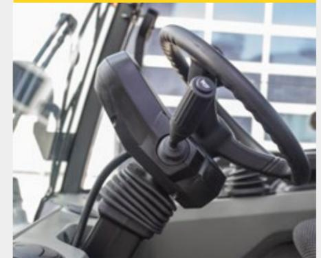
The optional tilt-adjusting steering column can be adjusted to suit the operator's requirements. The steering wheel consists of a high-quality, non-slip material. The steering column also includes a modern dashboard display with automatic blinker reset.
