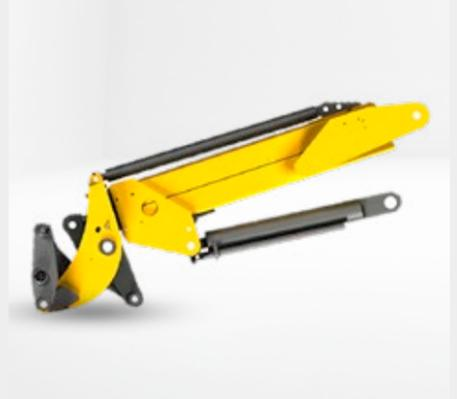
The view of the attachment is exceptional thanks to the compact modular design of the telehandler system. The advantages of Z-kinematics: in the case of equal size cylinders, dumping in a bucket creates a higher tearout force since pressure is applied to the piston side of the hydraulic cylinder when filling the bucket.
