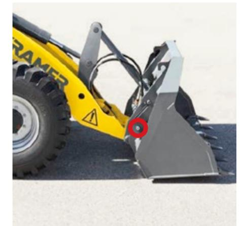
**Hydraulic quick-change system - The Kramer quickhitch system:** approach the attachment, pick up the attachment hydraulically from the operator's seat and lock it using the touch slide on the joystick. The lock cylinder is located outside of the pivot point of the quickhitch plate and is thus not in the contamination area.
