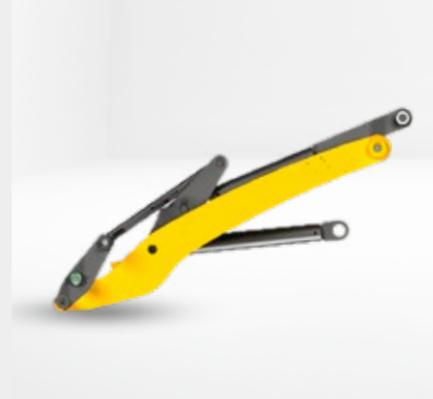
The parallel-guided loader unit ensures constant lift capacity and a safe operation in materials handling. Due to the tilt back angle of up to 45° and a tilt-out angle of up to 45°, the wheel loader does not lose any material in bucket application, even when it is very full, allowing for a complete emptying of the bucket.
