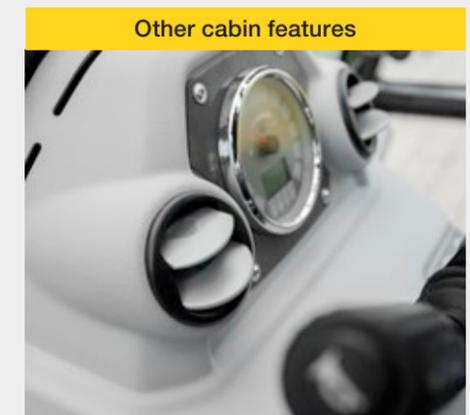
The powerful heater with window ventilation and heating nozzles in the footwell ensures comfortable working, even on cold days. A fully integrated air-conditioning system is optionally available. The combined brake-inch pedal allows for precise manoeuvring, even at high engine speed.
