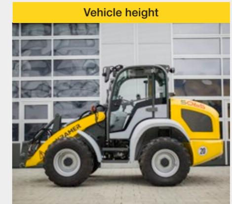
The machines offer the best conditions for low headrooms. All machines have an overall height of less than 2.5 m. The compact construction of the wheel loader 5050 enables easy transport on a 3.5 t trailer.
