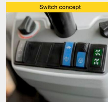
The respective functional group is very quick and easy to identify due to the colour-coded switches. Red = safety, green = hydraulics, blue = travel and grey = electrical system. This ensures the operator a convenient and safe operation without the risk of being confused. The result is increased working efficiency for the operator.
