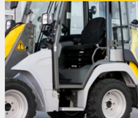
The wide entry includes additional steps, thus ensuring comfortable entry and exit. Two grab handles fixed to the cabin help the operator to get in and out of the cabin safely. The cabin door can also be opened through 180 degrees and locked to the machine.
