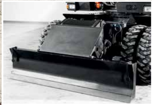
Large blade cylinder cover offers greater protection.
