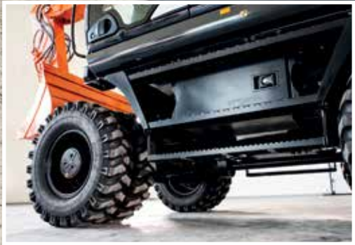
High ground clearance reduces damage from obstacles.
